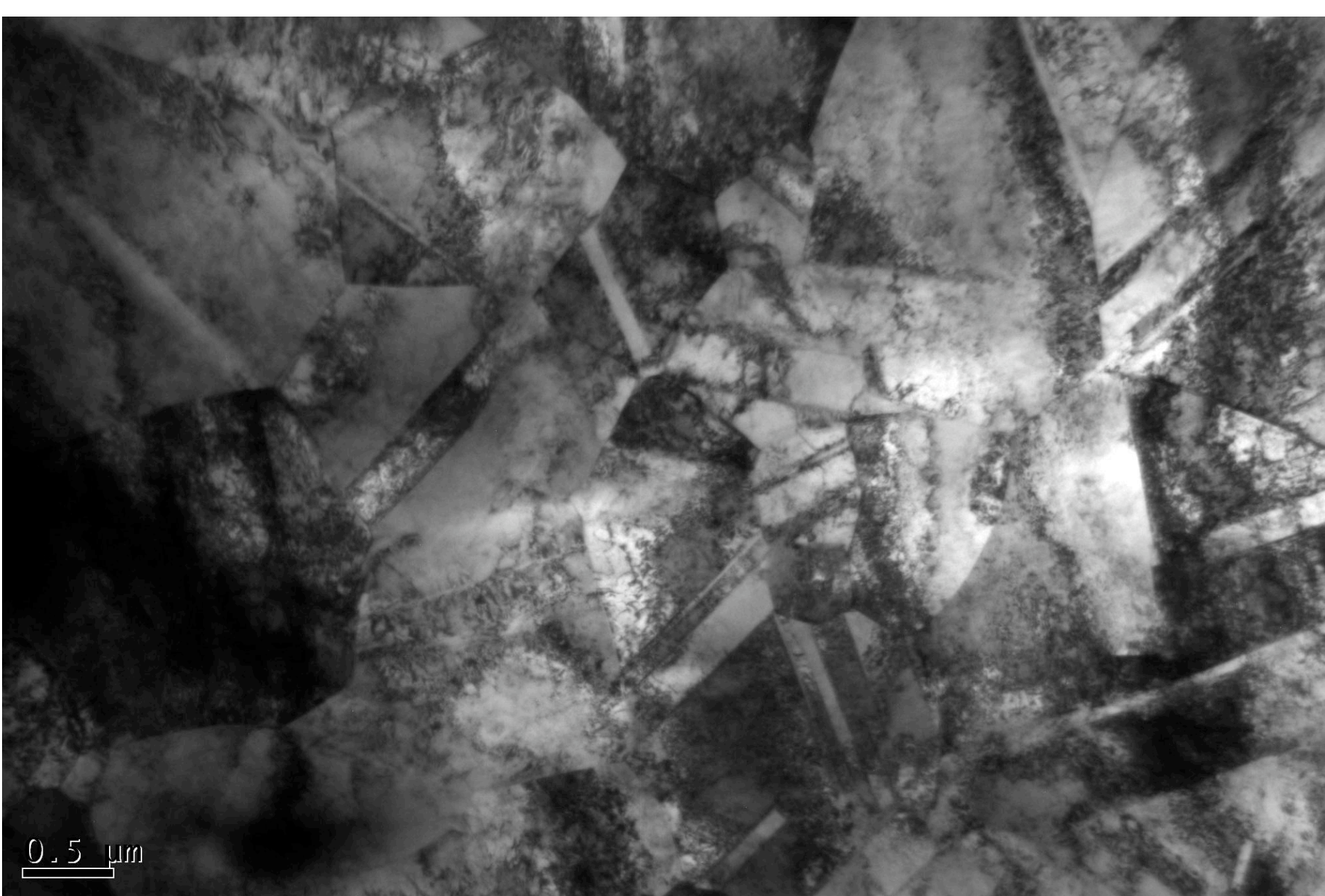
Cu-773K pre-annealed matrix (high density of dislocation-network)
