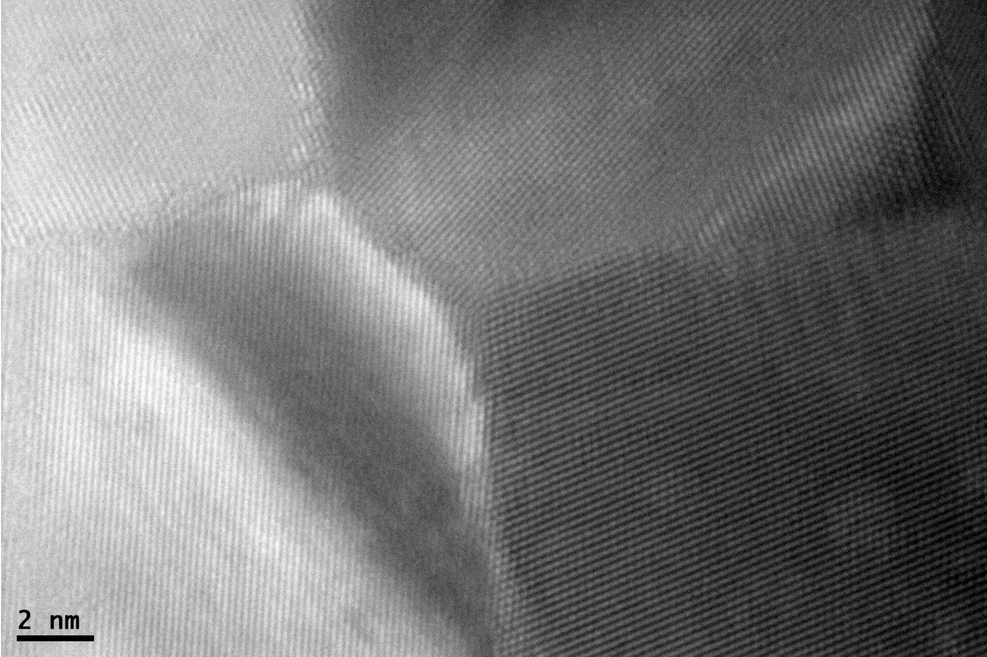
Grain boundary width \sim 1\text{nm} , with various crystallography orientations
