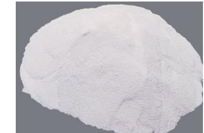
**Powders are mixed homogeneously through ball milling, pressed and annealed at 1400 °C to reach the theoretical density**
